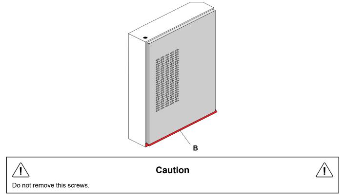
Keep this angles to eventually lift the machine. Block the screws which maintained this angles.
