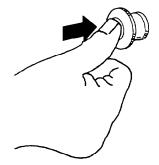
Release the emergency stop, by turning it clockwise only after checking what motivated this stop.
