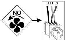
Check again the direction of the rotation of the fan then replace the hose and its collar.
