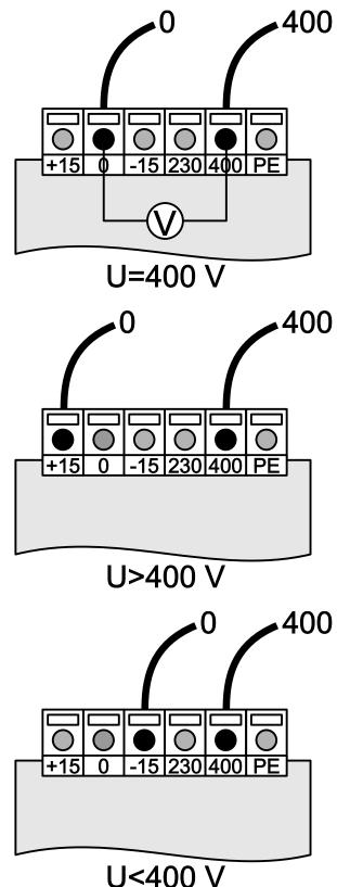
If the voltage is > 400 volts (example: 420/230 volts), connect threads to the transformer as indicated in the margin.
