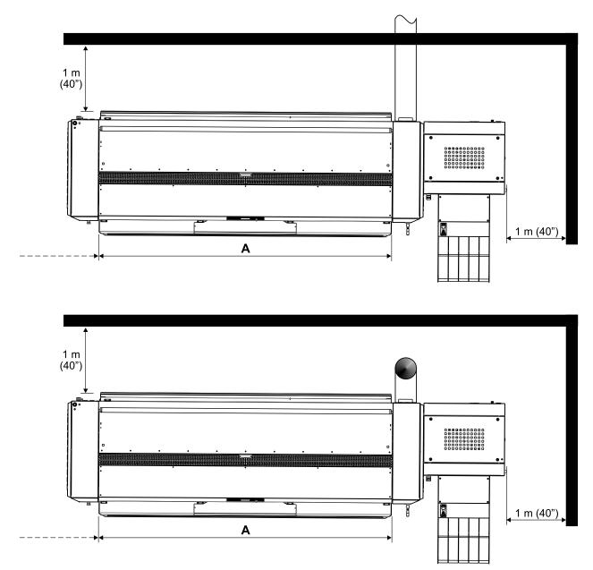
However, note that if you can, it is recommended that you should leave sufficient space for maintenance of the heating box to avoid having to move the machine (minimum length A on the left side).
